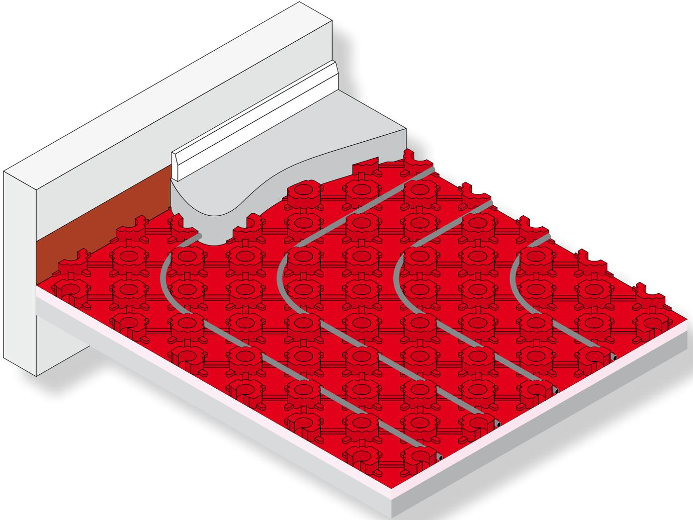
**Polypipe underfloor heating in solid or screeded floors incorporates the unique Polypipe screeded floor panel. The lightweight plastic floor panels nest for easy storage and carrying.**
