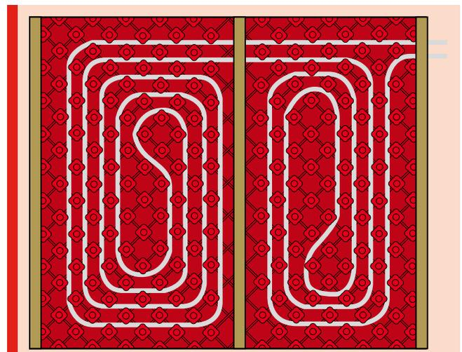
Individual circuits of pipe are then laid between each set of joists with care being taken to ensure the screed is completely dry prior to fitting the solid oak covering (see diagram below).
